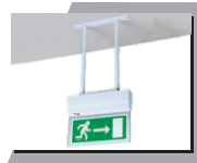
Model : PEL 108 E/M (SM) Lamp Type : 1 x 8W T5 FTL / 1 x 11W CFL Accumulator : Ni-Cd Battery Backup : 2 Hrs. Standard Pkg.: 4 pcs. Box size in mm : 380x300x340
