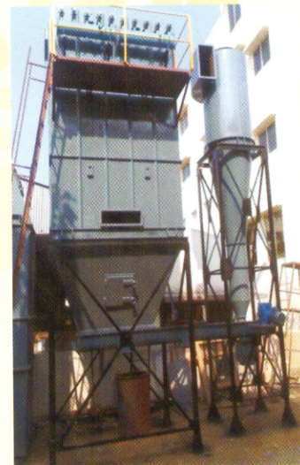
BAG FILTER WITH CYCLONE DUST COLLECTOR SYSTEM
